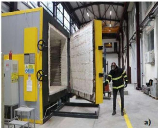
Fig. 3 Test furnace and application of high-temperature effect
