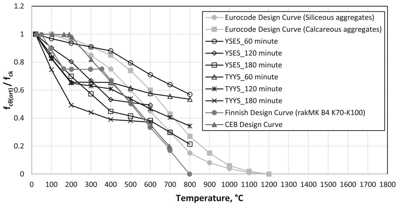
Fig. 11 Comparison of design curves and experimental strength loss curves
