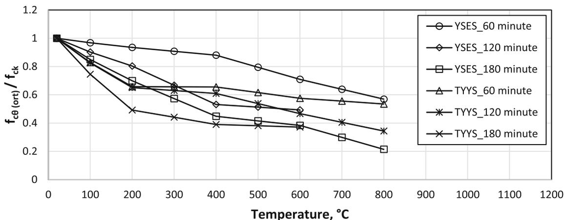
Fig. 9 Variation of compressive strength with temperature.  $f_{ck}$ ; Compressive strength of reference standard cylinder concrete specimen not exposed to high temperature
