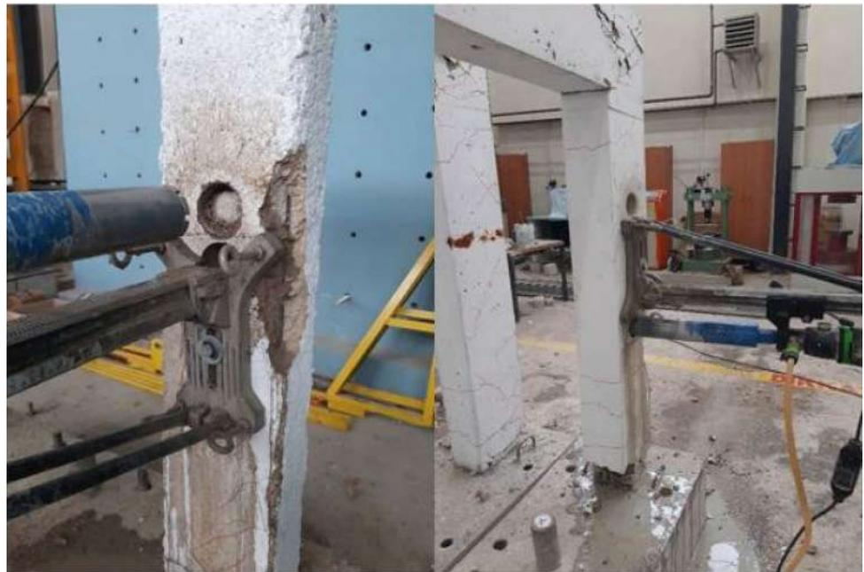
to high temperature and 70 mm × 105 mm cylinder concrete core specimens taken from reinforced concrete frame test members subjected to cyclic load effect after high temperature, the compressive strengths of the cylinder concrete core specimens were adjusted by multiplying the size effect correction factor specified in ASTM C42 [41] by 0.96.
