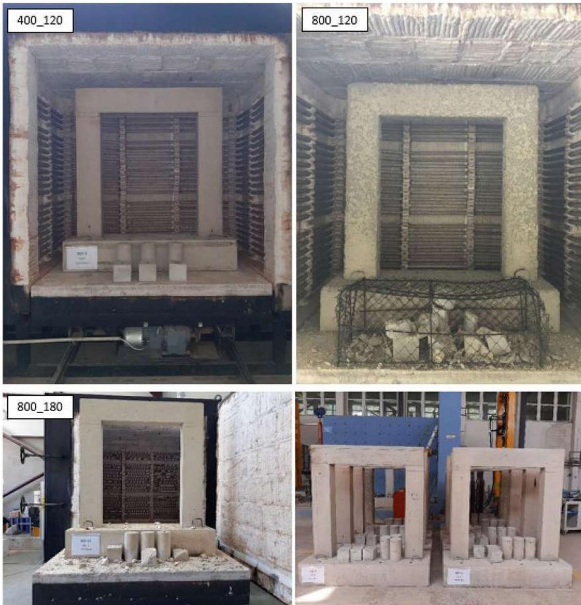
**Fig. 4** Concrete specimens subjected to high-temperature effect
