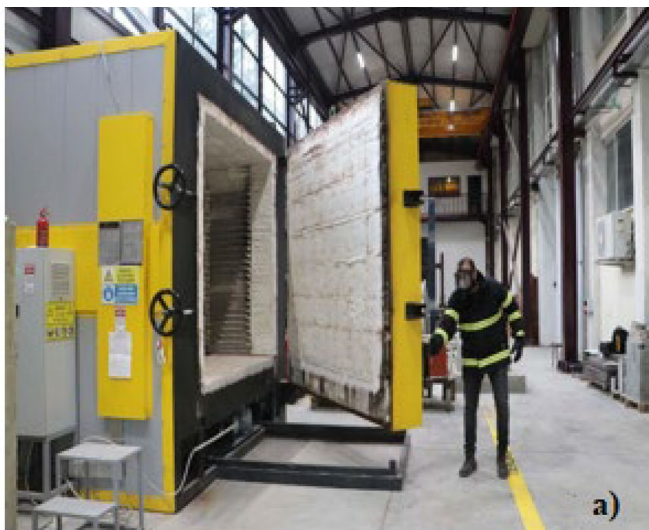
Fig. 3 Test furnace and application of high-temperature effect
