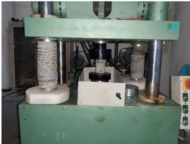
Fig. 8 Determination of compressive strength of concrete core samples.
