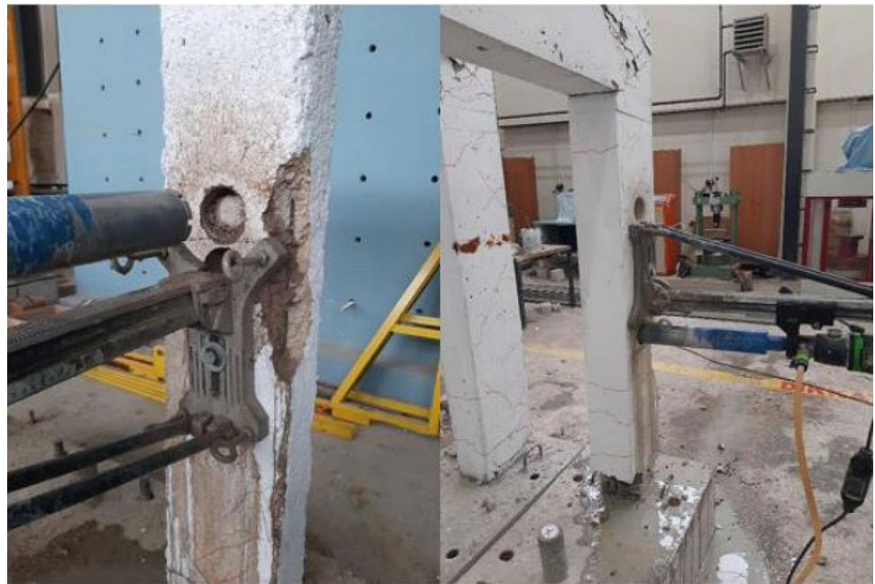
Fig. 7 Core sampling from test elements
