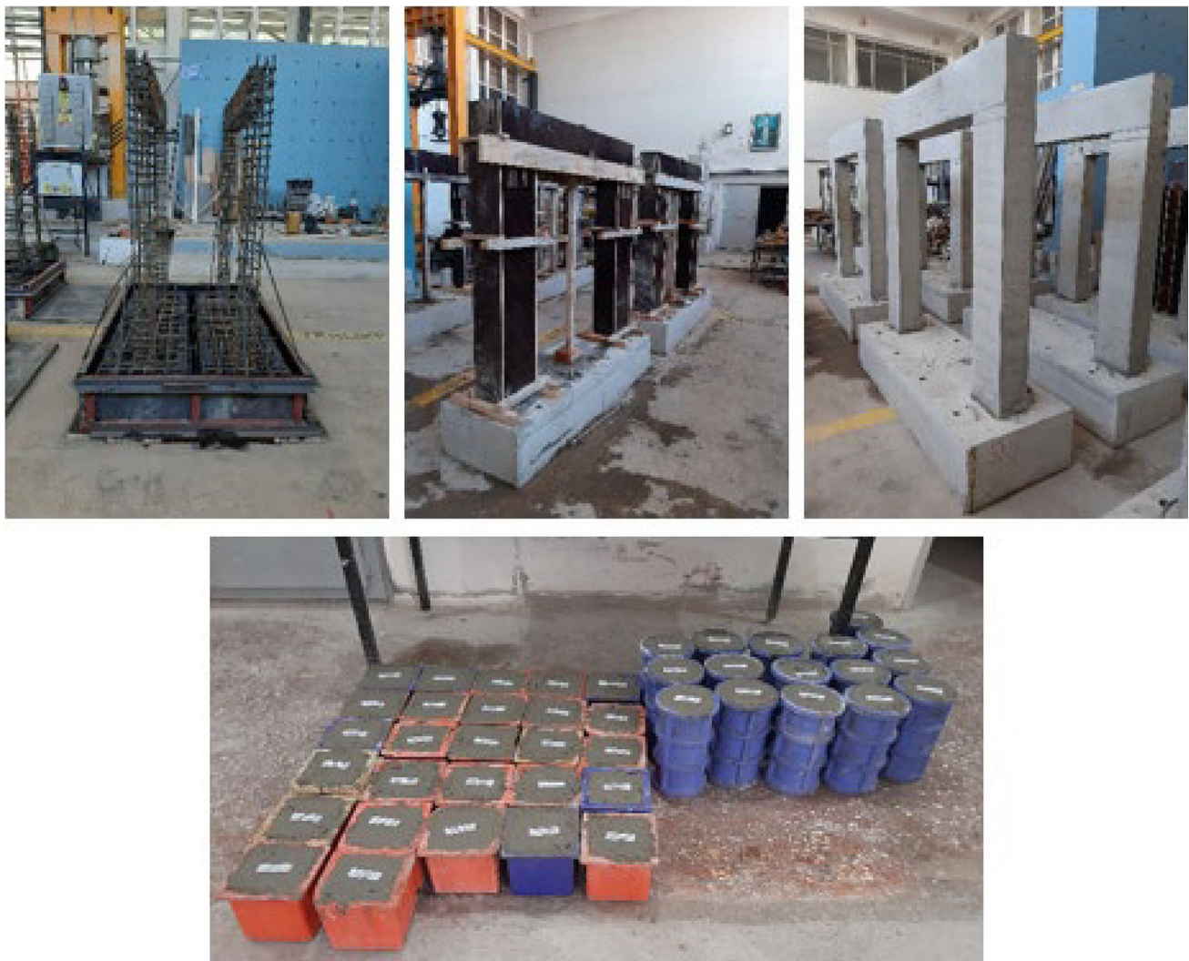
Fig. 2 Reinforced concrete frame test elements and concrete specimens
