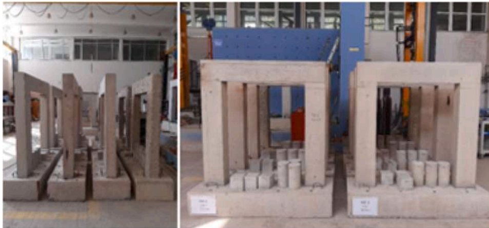
Fig. 6. Test specimens exposed to the high-temperature effect and concrete sample examples.
