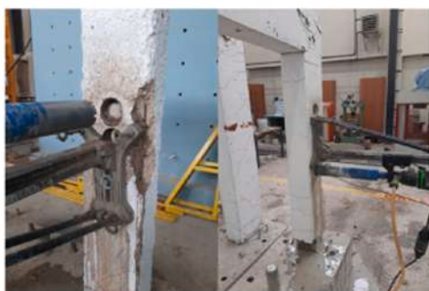
Fig. 16. Core sampling process from test elements.
