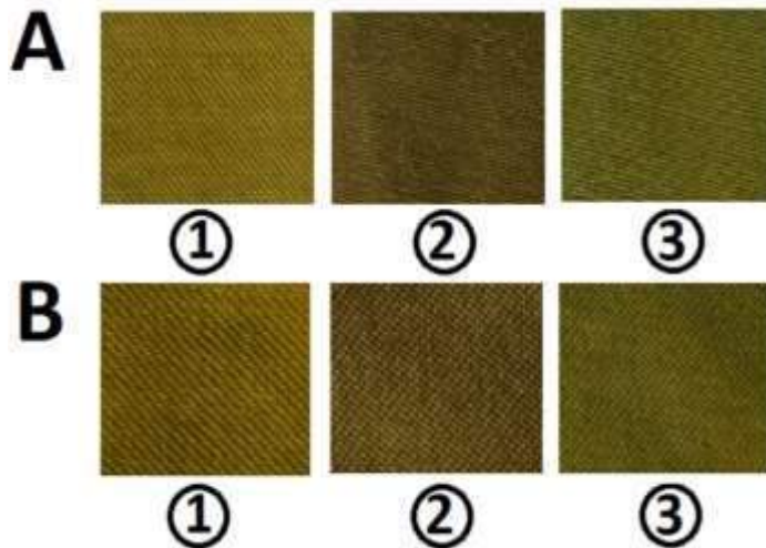
Figure 2. Natural dyed wool fabric with P. cognatum , (A) 25% natural dye concentration, (B) 50% natural dye concentration. Mordanting processes (1) 20% KAl(SO_4)_2 \cdot 12H_2O , (2) 3% FeSO_4 \cdot 7H_2O (3) 5% CuSO_4 \cdot 5H_2O
